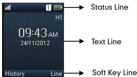
The LCD screen is divided into three parts: status line, text line and soft key line.
