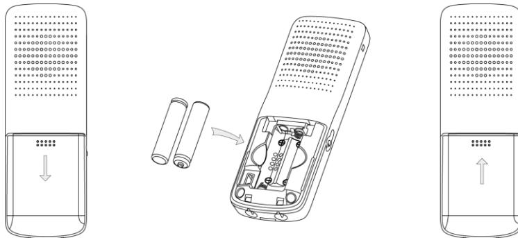
**Note** Do not short-circuit the batteries, as short-circuiting the terminals may damage the batteries or the handset.
